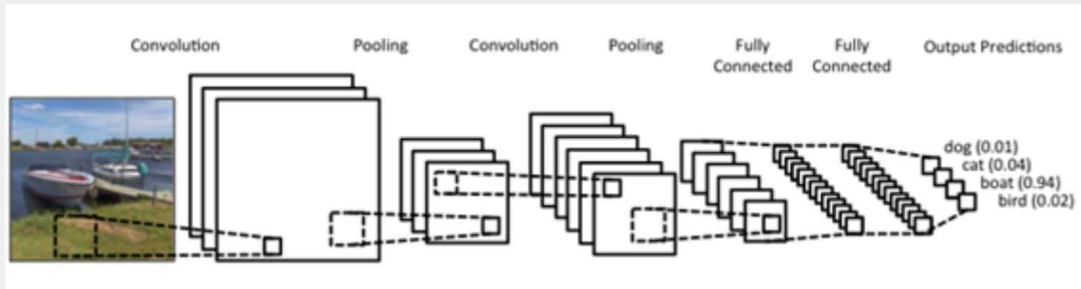
**Figure 1:** Example of CNN used for an image classification task
