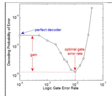
Figure 1 Stochastic resonance in Gallager B decoding algorithm. The memory element error rate is 0.006.
